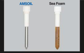
\*Based on independent third-party testing of AMSOIL Gasoline Stabilizer obtained July 1, 2022, and Sea Foam Motor Treatment purchased June 30, 2022, in a modified NACE TM0172 using synthetic sea water per ASTM Dö65B. \*All trademarked names and images are the property of their respective owners and may be registered marks in some countries. No affiliation or endorsement claim, express or implied, is made by their use.
